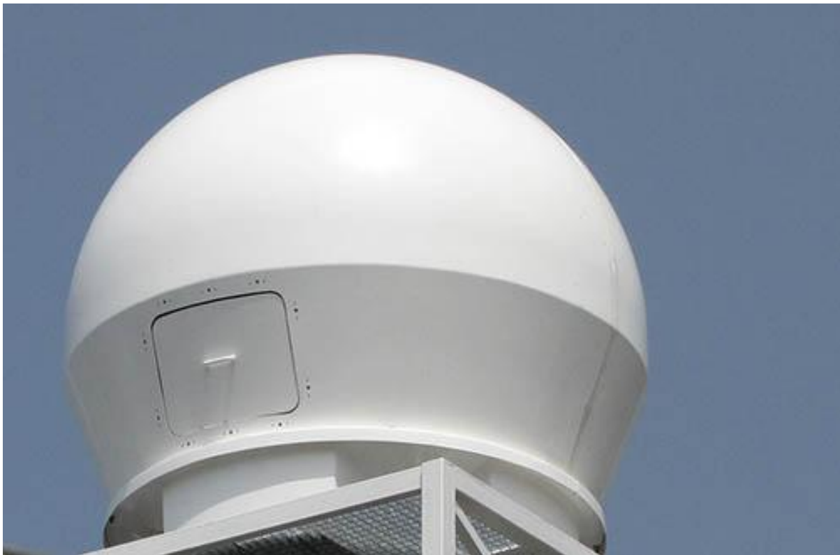
Dartcom 1.5m parabolic dish antenna and rotator inside glass-fibre radome.
