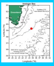
With a hydrographic mooring in the centre of the **Irminger Sea** profiles of temperature, salinity, and derived properties were determined from 2003 to 2010
